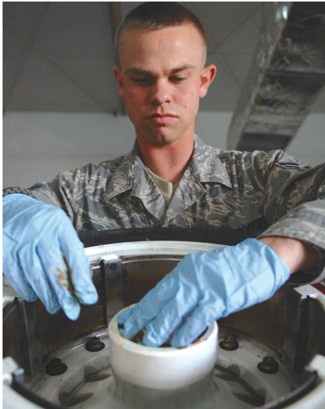
An Airman replaces retaining rings on an F-16 Fighting Falcon's main landing gear.
